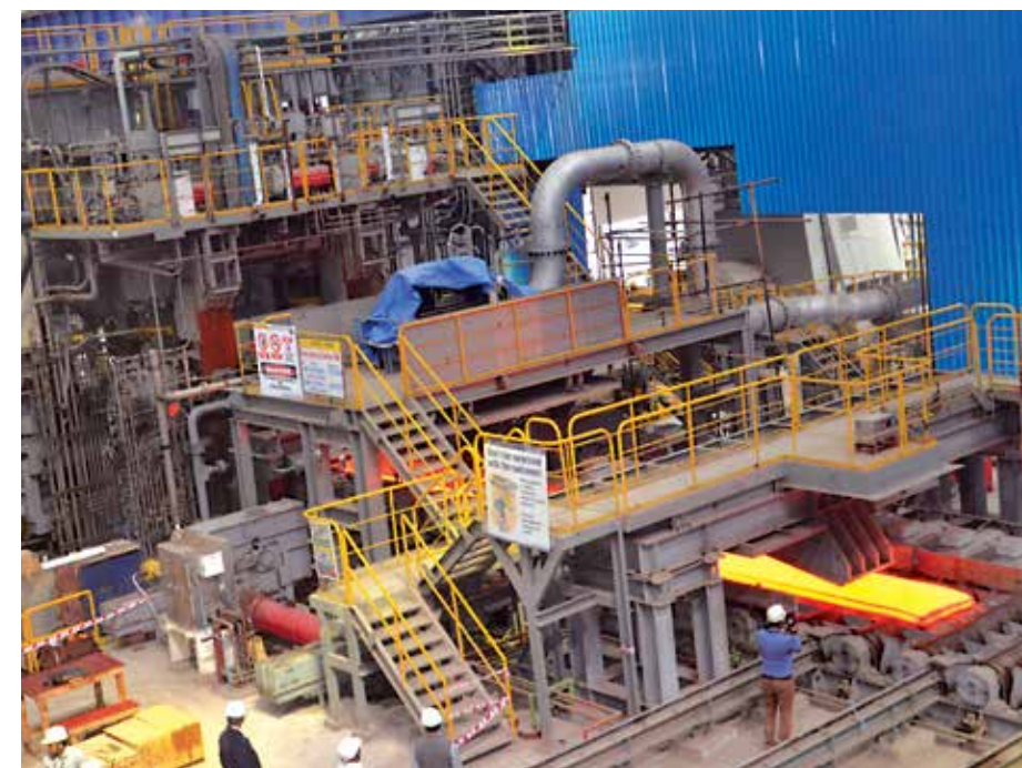
Hot slab being passed through the roughing mill
