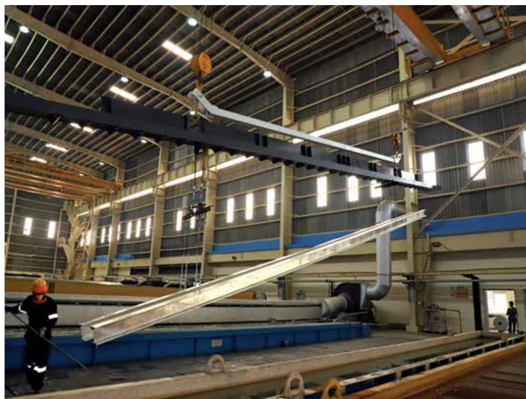
OHE fabrication and galvanizing facility at TL factory, Pithampur
