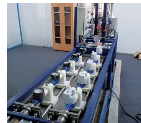
Testing of water meters
