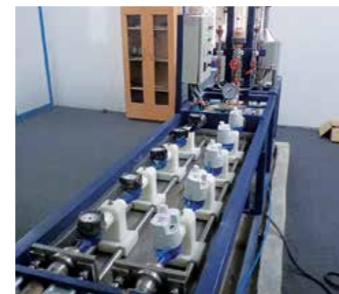
Testing of water meters
