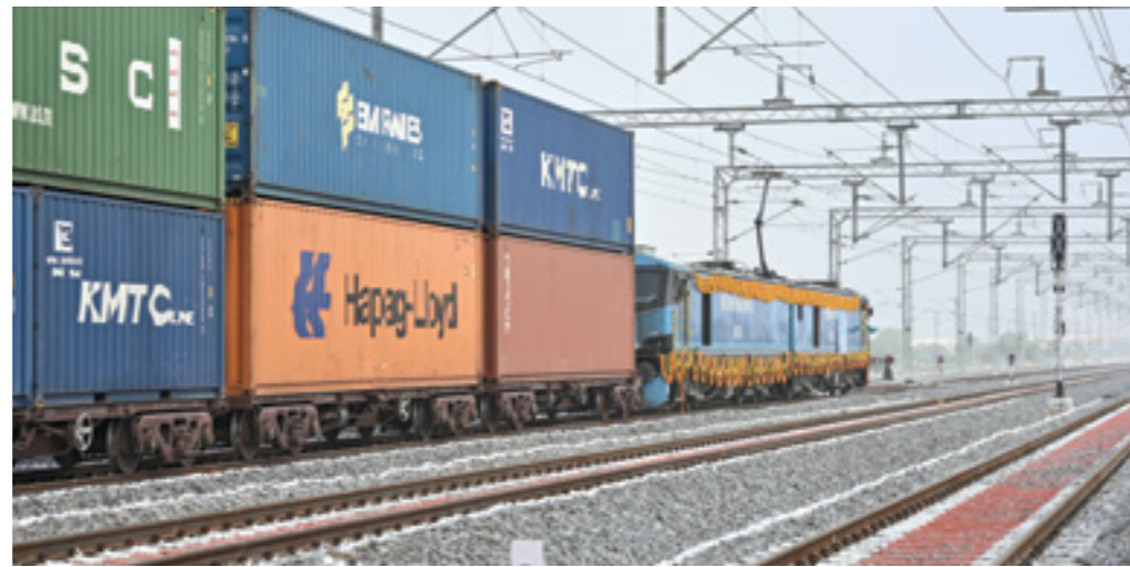
Heavy Haul Double Stack Container Rakes Powered by 12000 HP Electric Locos - WDFC CTP 1 & 2 sections in Regular Commercial Operation
