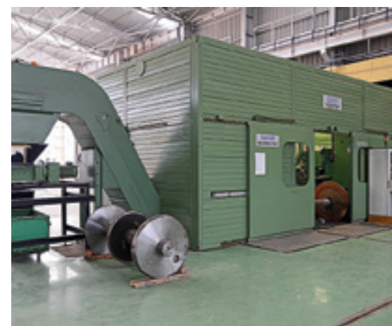
Wheel lathe at Wagon repair shop - Jhansi
