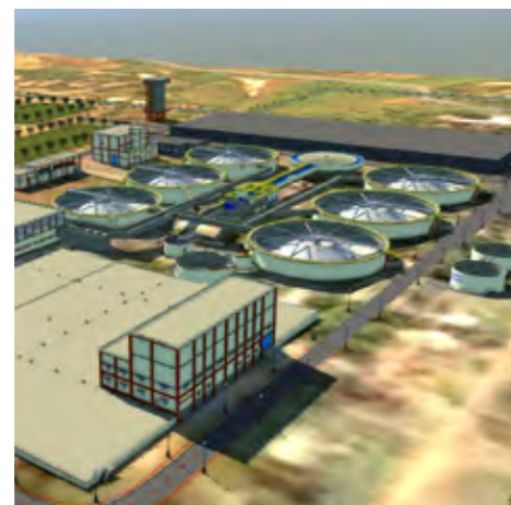
BIM Model of a Water treatment plant
